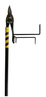
He added the unique mechanical concept of Skyridder, which uses a lamp post as the holding force to enable a special wire cutter compared to existing methods such as wire and pulley.
