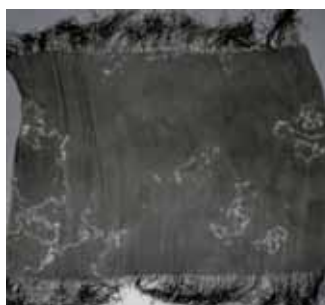
Figure 1: Microelectrode wire cloth produced
