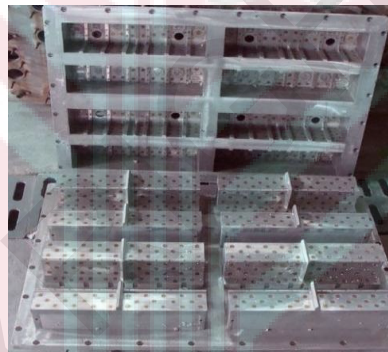
Figure 1.6 : Example of EPS moulding tools (PMPF CO., LTD)
