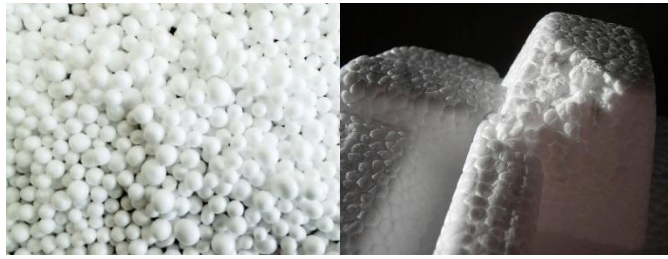
Figure 1.2 : Expanded Polystyrene (EPS) beads (CIGA et al., 2020)
