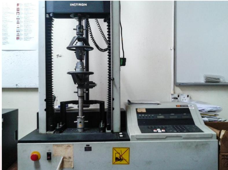
**Appendix A7: Tensile test conducted using Instron Universal Tester.**
