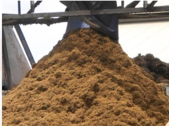
**Figure 2.8: Mesocarp fiber after oil extraction.**
