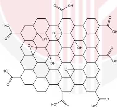
Figure 1.3: Chemical structure of graphene oxide. (Chakraborty & Hashim, 2018)
