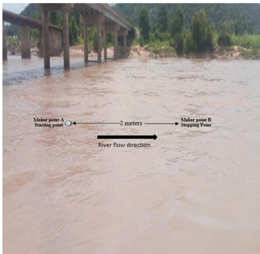
Figure 4. Measurement of water velocity data using Surface Floating Method.
