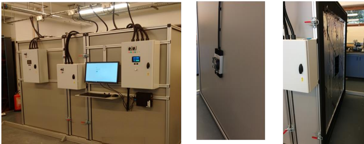
Figure 2. Clockwise: The constructed small calibrated hot box, the specimen area and the thermoelectric assembly unit for heating and cooling
