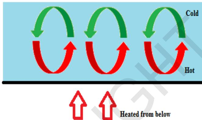
**Figure 1.2: Thermal convection in a fluid.**
