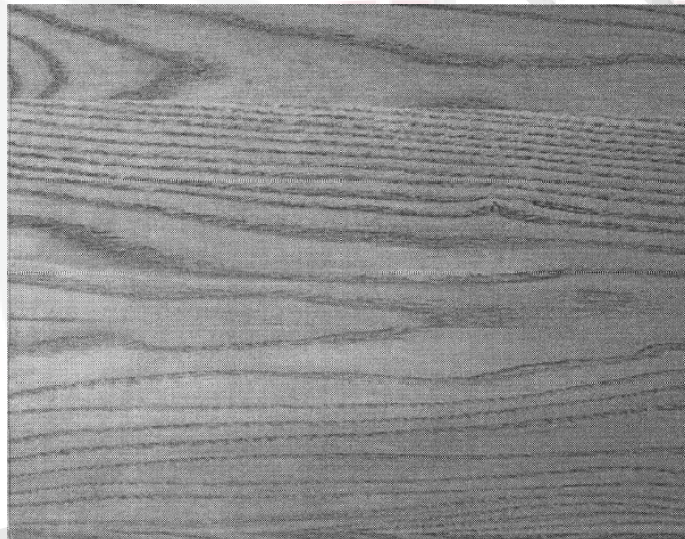
Figure 1.8: Wood is a very good example of a porous medium which exhibits a strong anisotropy (Source: Straughan, 2008)
