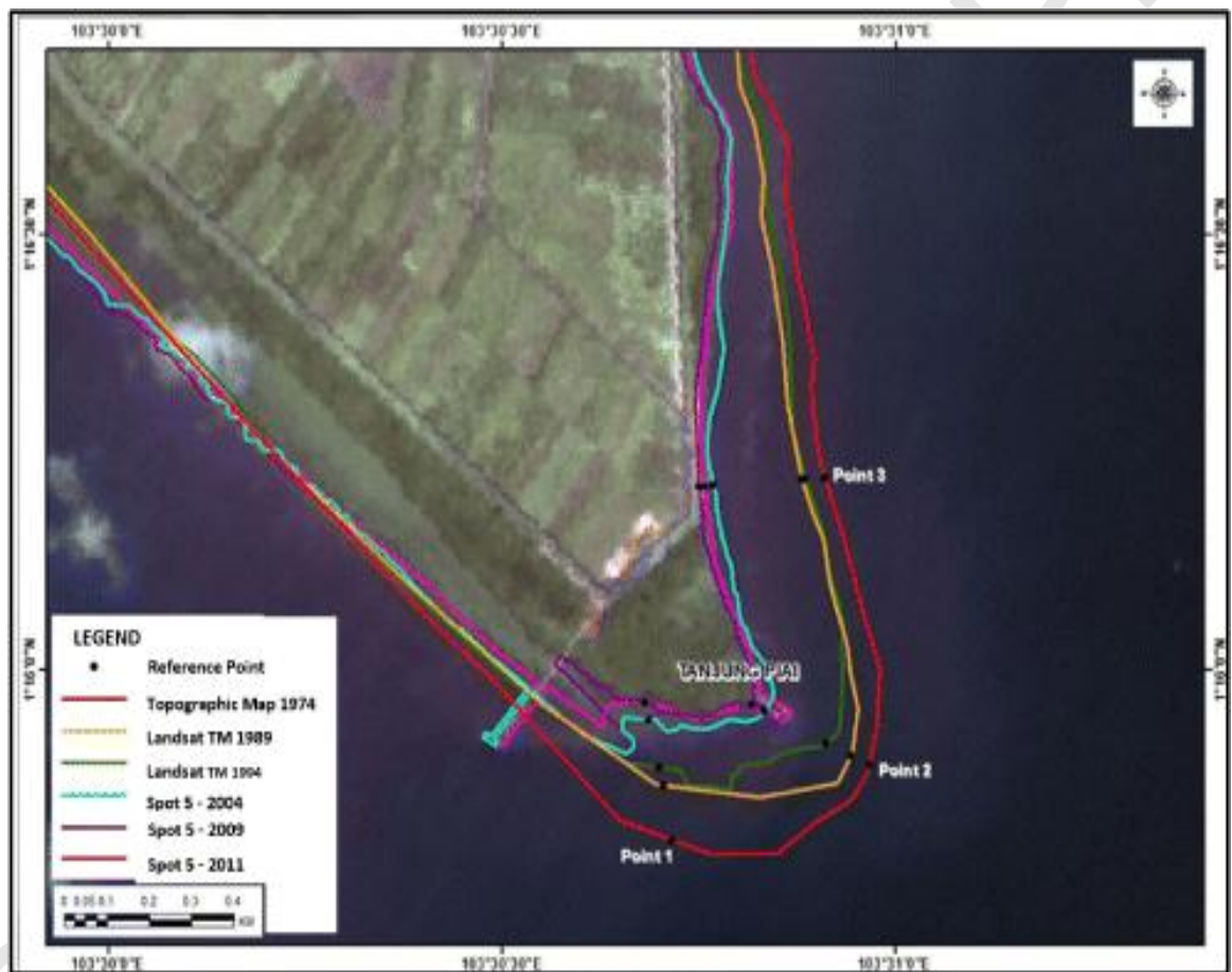
Figure 1.1: Shoreline changes due to coastal erosion at Tanjung Piai from 1974 to 2011 (DID, 2013)
