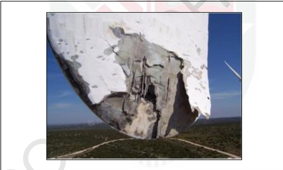
**Figure 1. 2: Lightning damage due to lightning strike (D. Li et al., 2015)**
