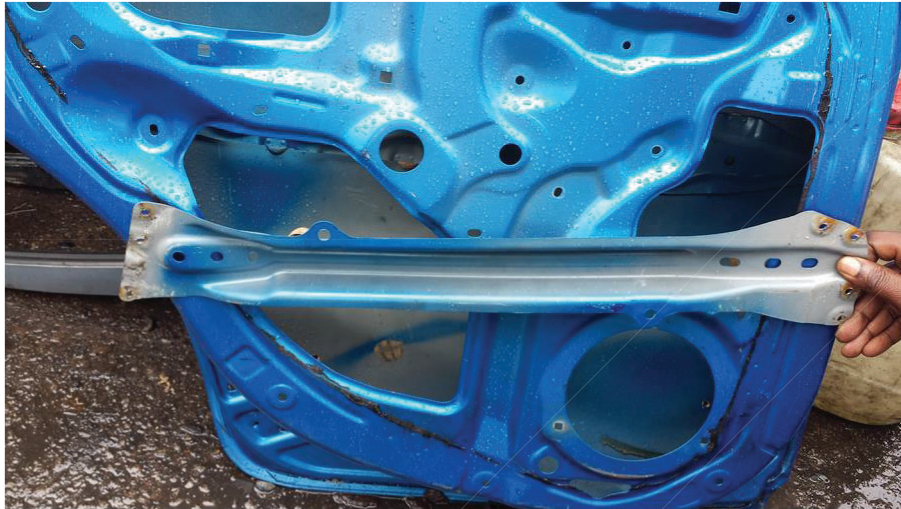
Figure 1.1: Side door impact beam for car occupants' protection
