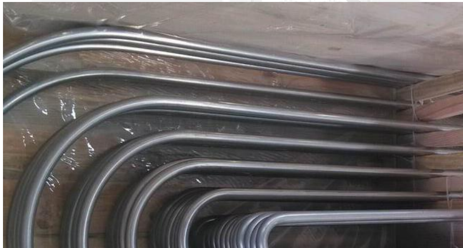
Figure 1.1 : Using Bend tubes in the heat exchangers (Vasu et al. 2012)
