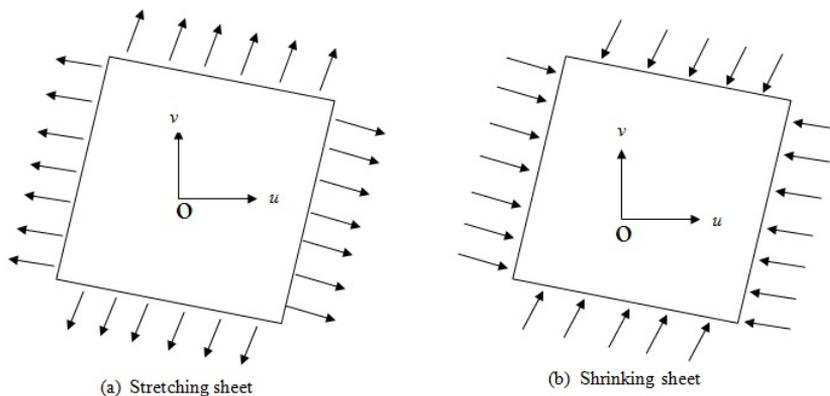
**Figure 1.8: Physical model and coordinate system for flow towards shrinking sheet**
