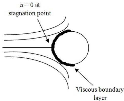
**Figure 1.4: Physical model for flow at Stagnation point**
