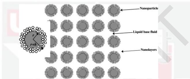
**Figure 1.5: Physical model for Nanofluid [Kakaç and Pramuanjaroenkij (2009)]**
