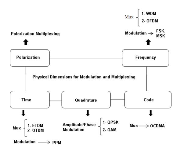
Figure 1-2: Physical dimensions that can be used for modulation and multiplexing in optical communications [2, 6, 7, 23-25].
