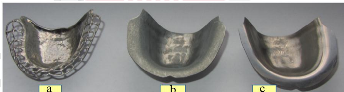
Figure 1.3 : Some of the medical parts produced by ISF: a) Cobalt-chrome alloy (cast) b) EN DCO4 (ISF) and c) EN X6r17 (ISF) (Milutinovića et al. , 2014)
