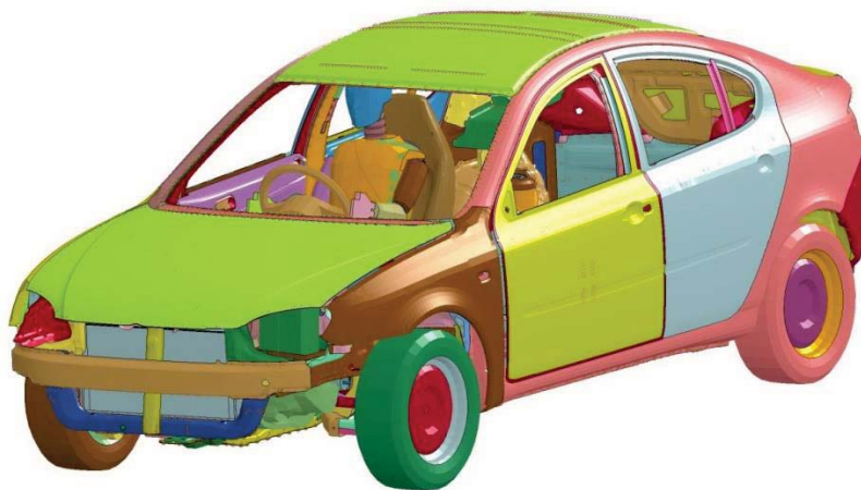
Figure 1.4: Vehicle model designed using CATIA
