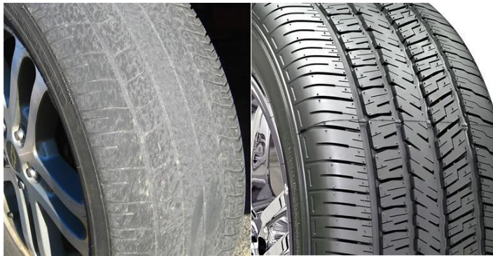
Figure 1.1. Full and Effective Contact Areas, Close-up View of the Void Areas
