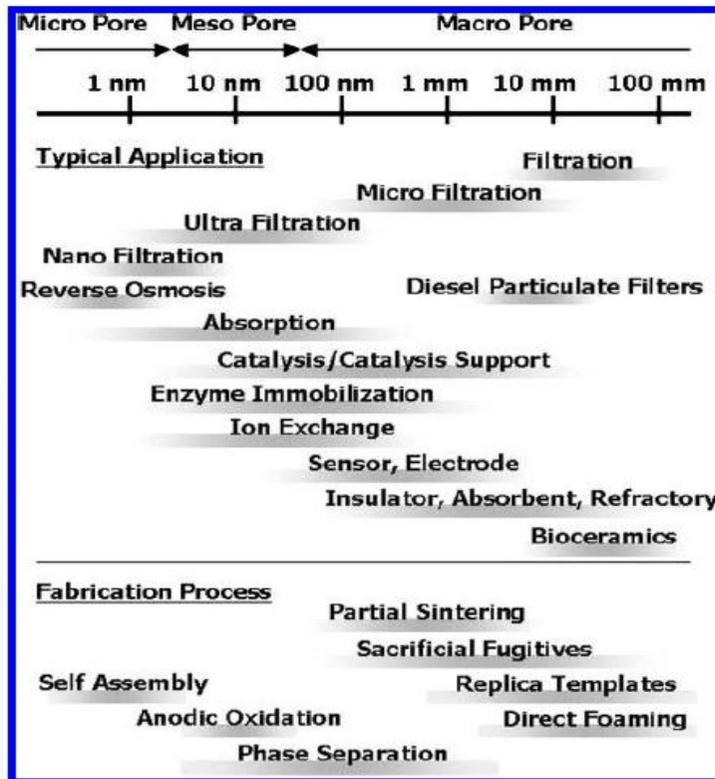
**Figure 1.1: Classification of porous ceramics according to pore size, applications, and fabrication methods (Ohji and Fukushima, 2012)**
