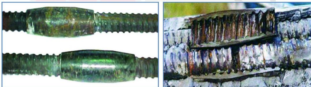
**Figure 1.3 : Illustrate the cable couplers before and after corrosion**
