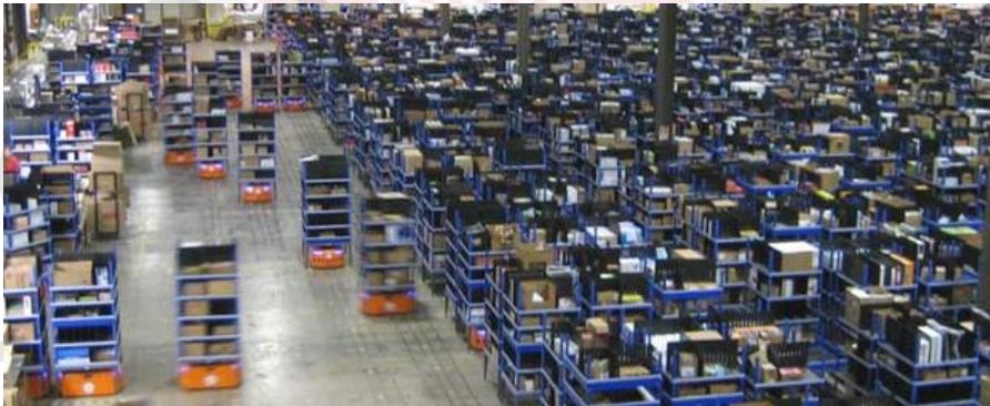
Figure 1.1: Mobile multi-robots in automated warehouse operations [4].
