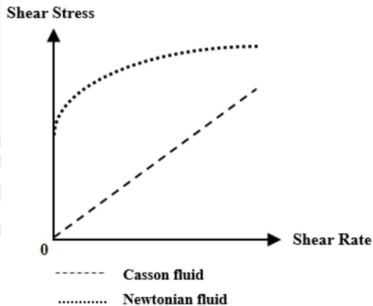
**Figure 1.3 : Rheogram of a Newtonian and Non-Newtonian fluid**
