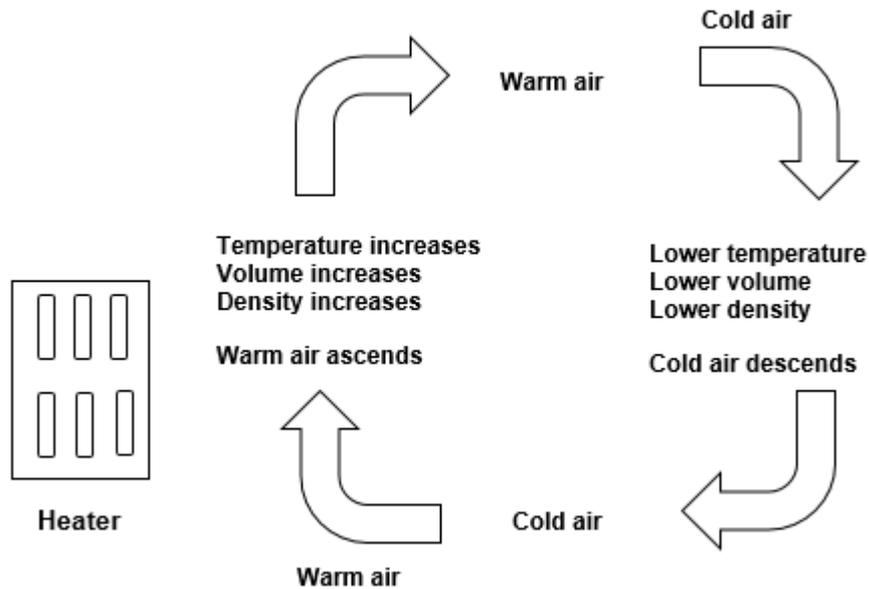
**Figure 1.2 : Demonstration of convection due to a heater in accordance with ideal gas law**
