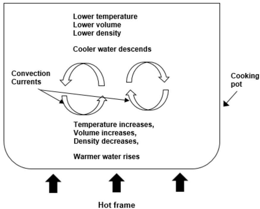
**Figure 1.1 : Convection circulation in a water heated in cooking pot in accordance with ideal gas law**
