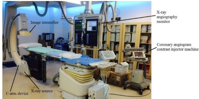
Figure 1.4: A typical x-ray angiography suite setup (Taken from UiTM Medical Center).
