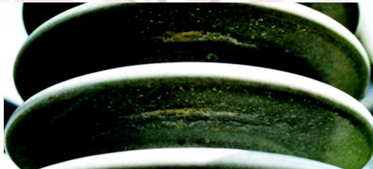
Figure 1.2. Surface of semi-conducting glazed insulator after one year long exposure to DC voltage in a marine environment [4]
