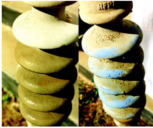
Figure 1.1. Appearance of water presence on bare and RTV-coated porcelain insulators contaminated with cement [4].
