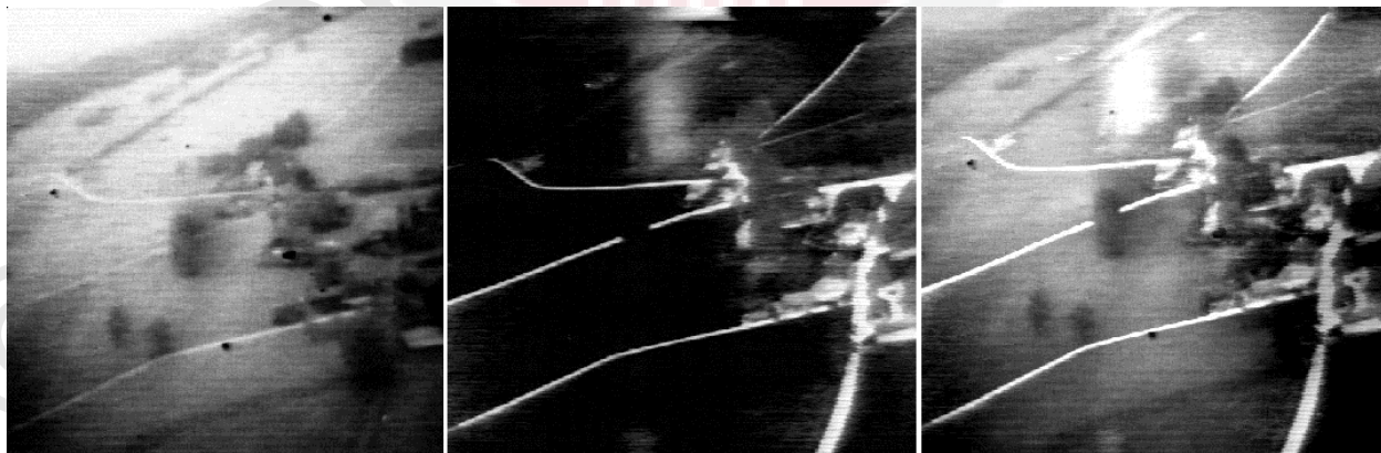
Figure 1.2: Image Fusion of digital camera (left image) and infrared camera (center image) with the output (right image) aimed for better navigation (Pajares and de la Cruz (2004)
