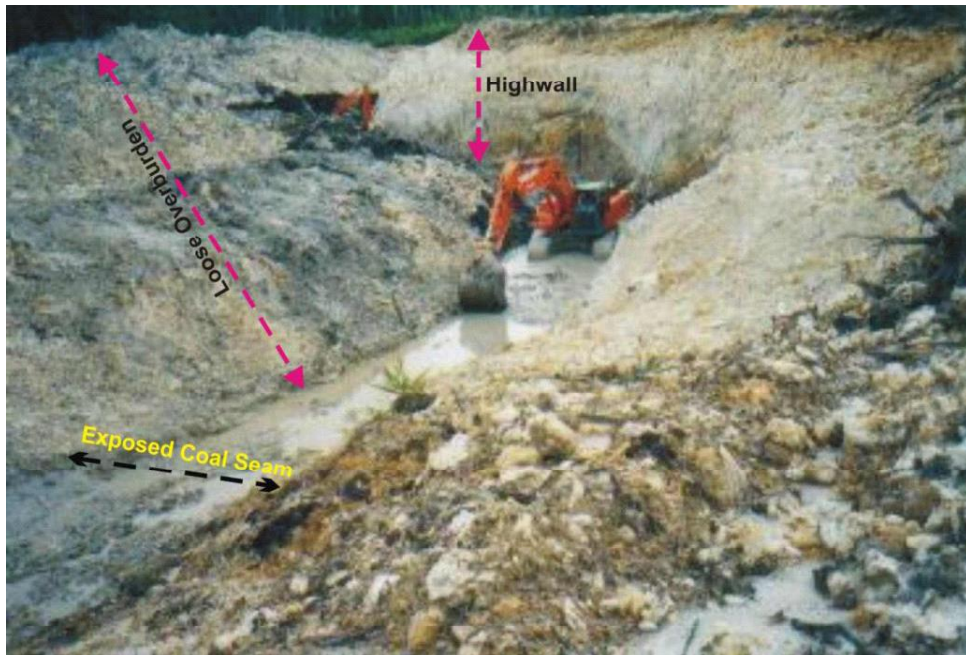
Figure 1.1. Exposing the coal seam and piled up overburden creating unstable high wall
