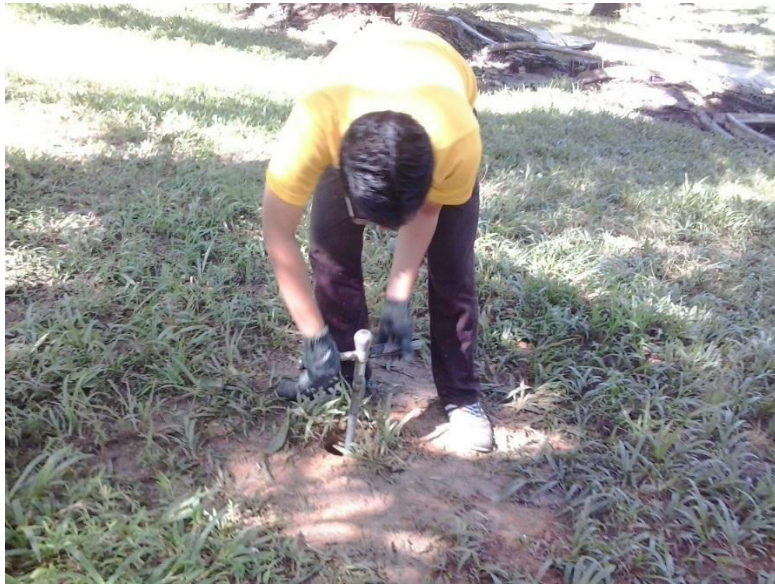
Appendix 1: Soil sampling by using auger.
