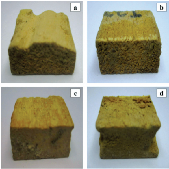
Figure 25 Sesenduk wood after 4 weeks of exposure to Coptotermes curvignathus Holmgren: (a) untreated sesenduk; (b) treated using 20% PF concentration; (c) treated using 15% PF concentration; and (d) treated using 10% PF concentration (Nabil et al. , 2016).
