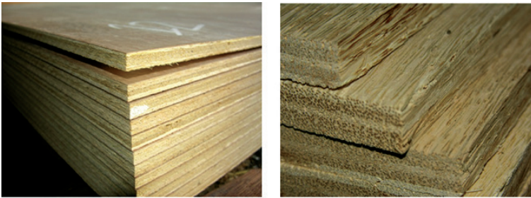
Figure 7 Oil palm veneers are used for plywood (left) and LVL (right) production
