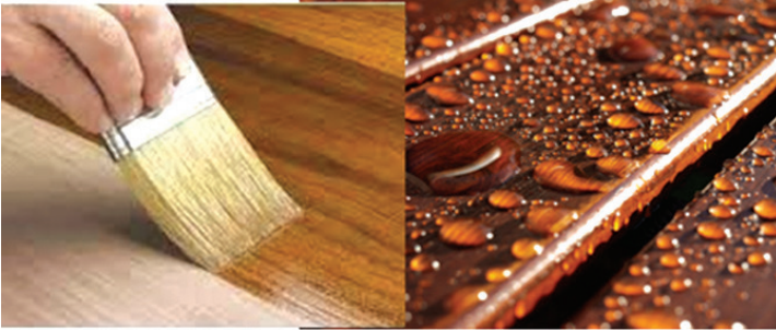
Figure 11 Water resistant coating to reduce moisture uptake
