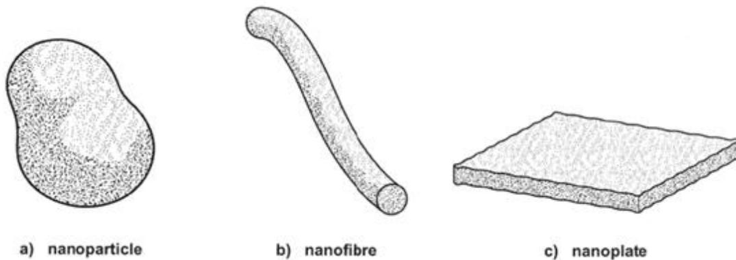
**Figure 1.2: Illustration of possible nano-objects as defined. a) Nanoparticle: b) Nanofibre c) Nanoplate (Image adapted from ISO/TS 27687: 2008(E) standard.)**
