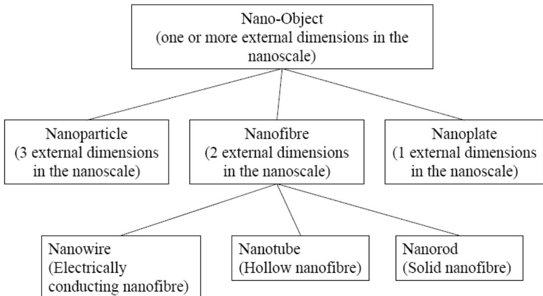
**Figure 1.1: Hierarchy of terminologies set as standard for nano-object (Adapted from ISO/TS 27687 : 2008 (E) standard)**
