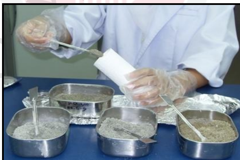
Figure A-2 Dried with anhydrous \text{Na}_2\text{SO}_4 & Transferred the sediments into cellulose thimble
