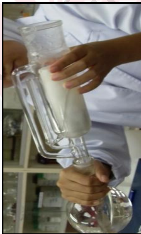
Figure A-3 Soxhlet Extraction with DCM for 10 hour
