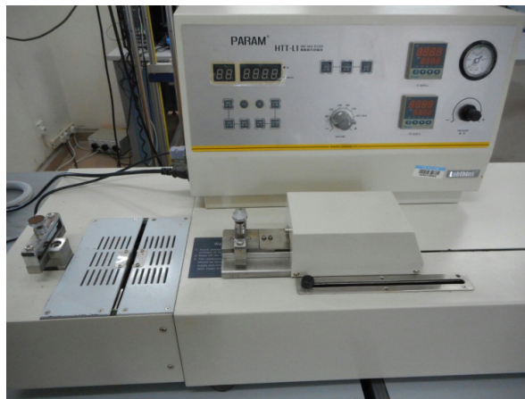
Figure 4. The Hot Tack Tester V2.04.1 was used for determining the tension limit of the two types of membrane
