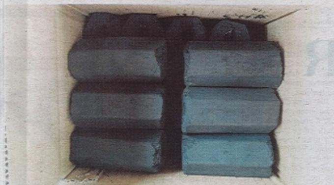
Biochar briquettes produced by the Biomass Microwave Carboniser.
