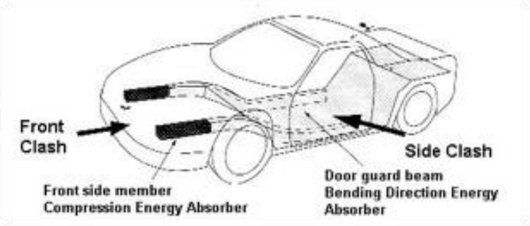
**Figure 1.2: Application of carbon fiber reinforced plastic as shock absorber for automobile [2].**
