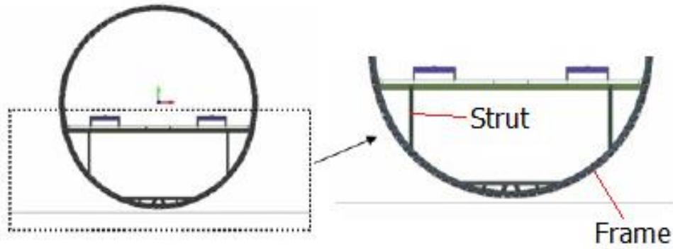
**Figure 1.1: Strut and frame structure of aircraft as energy absorber and support [1].**
