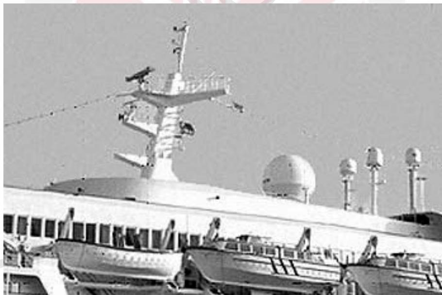
**Figure 1.5: Radome-enclosed SATCOM antennas. [11]**
