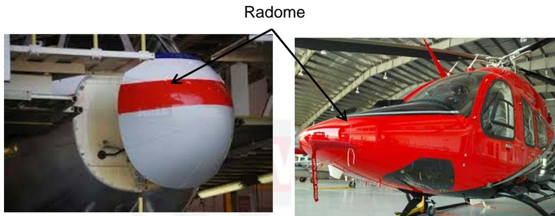
**Figure 1.6: Examples of aircraft radome. [12,13]**
