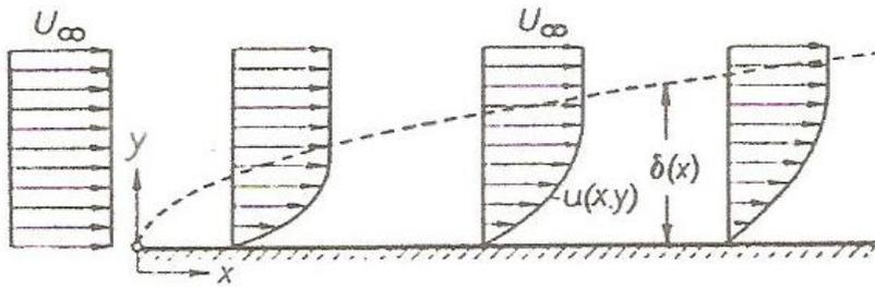
**Figure 1.1. Boundary layer on a flat plate in parallel flow at zero incidence (Schlichting, 1979)**
