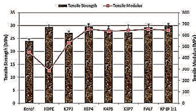
Figure 9. The tensile properties of hybridised kenaf/pineapple leaf fibre (PALF) at varying fibre proportions (Aji et al., 2013)
