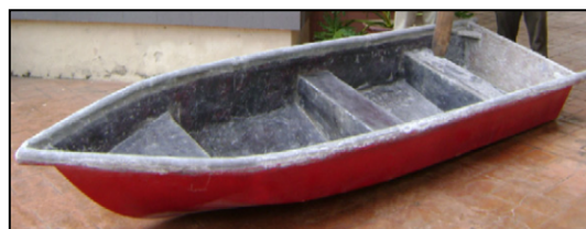
Figure 10. Mini boat made from hybrid sugar palm fibre with glass fibre reinforced unsaturated polyester composites (Ishak et al., 2011)
