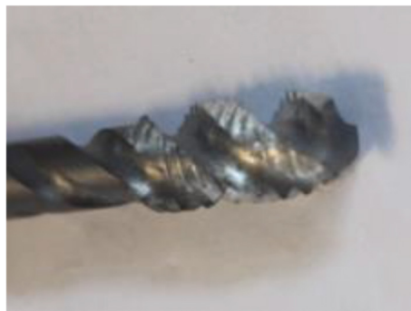
Figure 9. Aluminium stuck between the cutting edges of the tap
