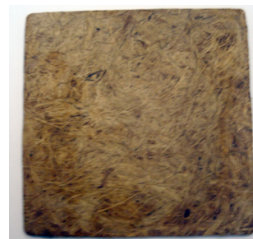
Figure 15. Environmentally-friendly composite from EFB fibres and binding agent from potato)
