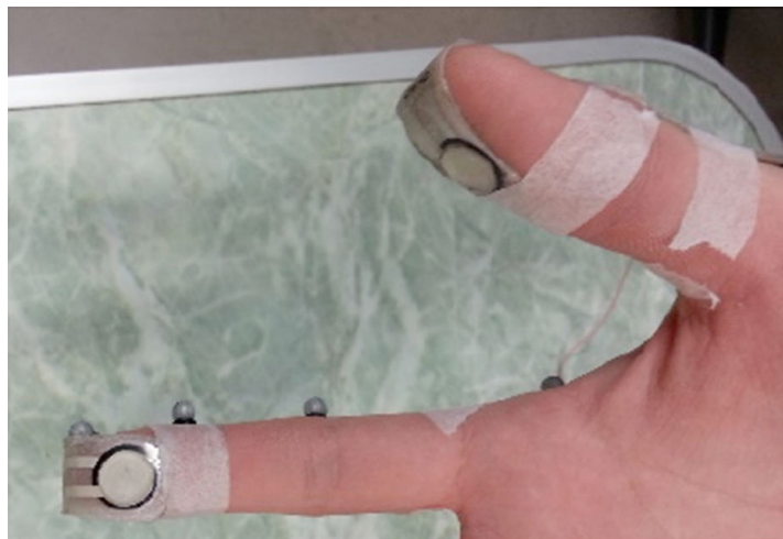
Figure 3. Flexi-force sensor position
