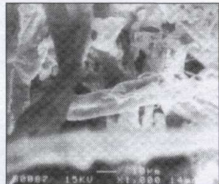
Plate 4: Recovered Malaysian fibre 1000X
