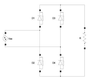
Figure 1. Single phase diode bridge rectifier circuit model.
