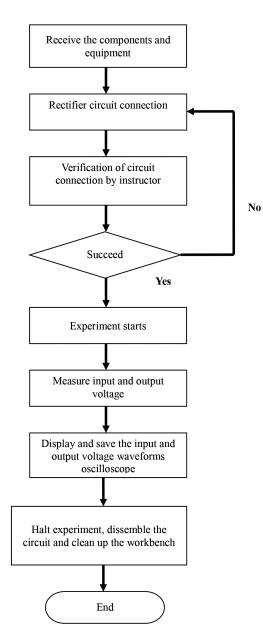
Figure 3. Flow chart of single-phase diode rectifier circuit experiment.
