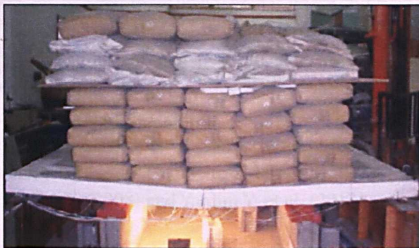
Figure 15 Simple performance test demonstrates the strength of the proposed system
