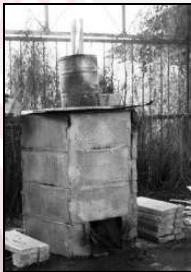
Figure 2.4a: A closed 200kg steel barrel kiln in Institute of Advanced Technology (ITMA), University Putra Malaysia (Rebitanim et al., 2013).
