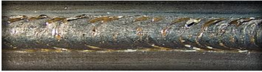
(a) A good weld
