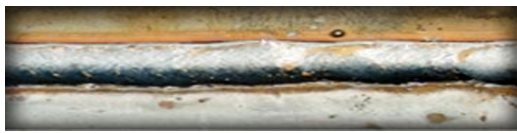
(b) Voltage Too Low
