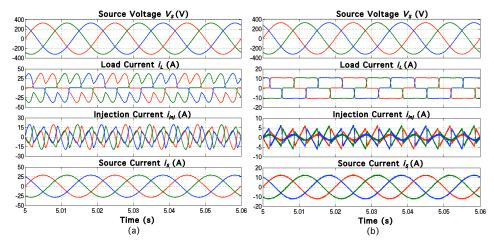
Figure 4. Simulation results of SAPF with effort-reduction FLC technique which include three-phase source voltage  $v_S$ , load current  $v_L$ , injection current  $i_{inj}$  and source current  $i_S$  for (a) capacitive, and (b) inductive loads
