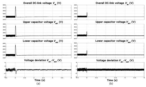
Figure 5. Simulation results of SAPF which include overall DC-link voltage  $V_{dc}$ , splitting DC-link capacitor voltages ( $V_{dc1}$  and  $V_{dc2}$ ) and neutral-point voltage deviation ( $V_{dc1} - V_{dc2}$ ) for dynamic state condition of capacitive to inductive load obtained using (a) conventional PI, and (b) proposed effort-reduction FLC techniques
