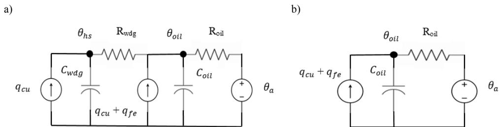
Figure 5. (a) Thermal heat transfer equivalent circuit; (b) Top-oil temperature thermal-electrical equivalent circuit
