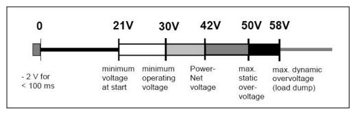
Figure 1.2. Power net voltage requirements for 42V (Traub, 1999).
