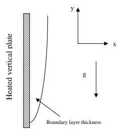
Figure 1.1: Schematic diagram of a vertical heated wall boundary layer.
