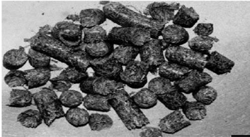
Figure 3. Picture of oil palm fronds pellet
