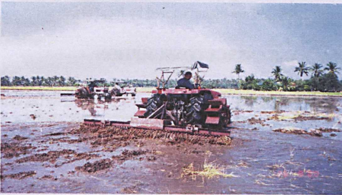
Figure 2 Land leveling by a tractor attached with cage wheels
